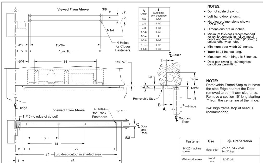
7900B Series Door Closers for 1-3/4" Thick Doors For Use on Doors Hung on 5" Wide Butt Hinges Maximum **Non Hold Open Installation** With Special offset Mounting in Wood Frame
