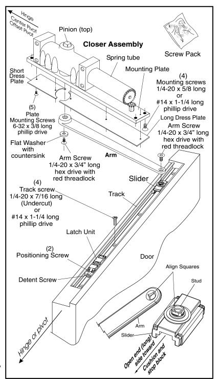
• Set Door opening angle With latch unit free, open door until slider and hold open unit are latched. Move door to hold open angle and secure latch unit by tighten 2 positioning screws with 1/8" hex wrench (supplied). Turn the detent screw clockwise to increase and counter clockwise to decrease hold open force with 3/16" hex wrench (supplied). Leave approximate 1" clearance from end of track for hex wrench to adjustment Detent. Release door.
