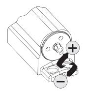
(Use 5/16" socket or adjustable wrench for Adjustment)
