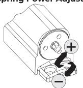
(Use 5/16" socket or adjustable wrench for Adjustment)
