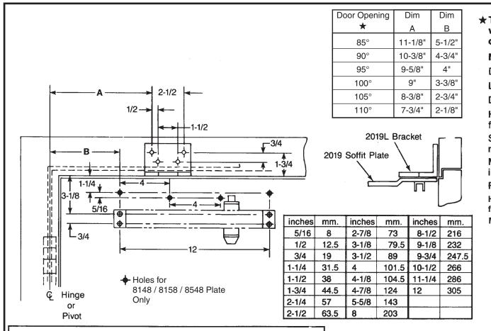
★ Template dimensions are for hold open/door stop within ± 2° of charted door openings. Doors may overtravel up to 5° beyond the rest position.
