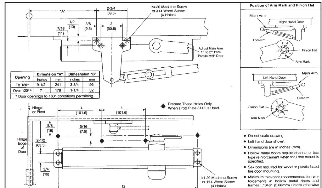
P8000 Series Door Closer for Narrow Stile Door With or Without 8148 Drop Plate Parallel Non-Hold Open Low Profile Arm Application P8180, P8380, and P8580 Sizes 1 Thru 6
