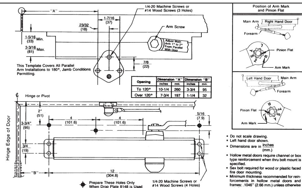
**P8000 Series Door Closer** Parallel Arm Application With 2018 For Between Doors With or Without 8148 Drop Plate
