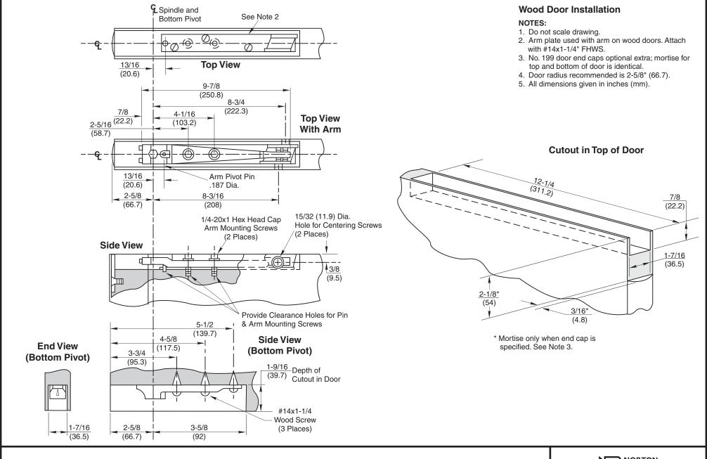
AW608 Series Overhead Concealed Door Closer Double or Single Acting for Aluminum Frame & Wood Door Center Hung, End Loading NORTON RIXSON ASSA ABLOY
