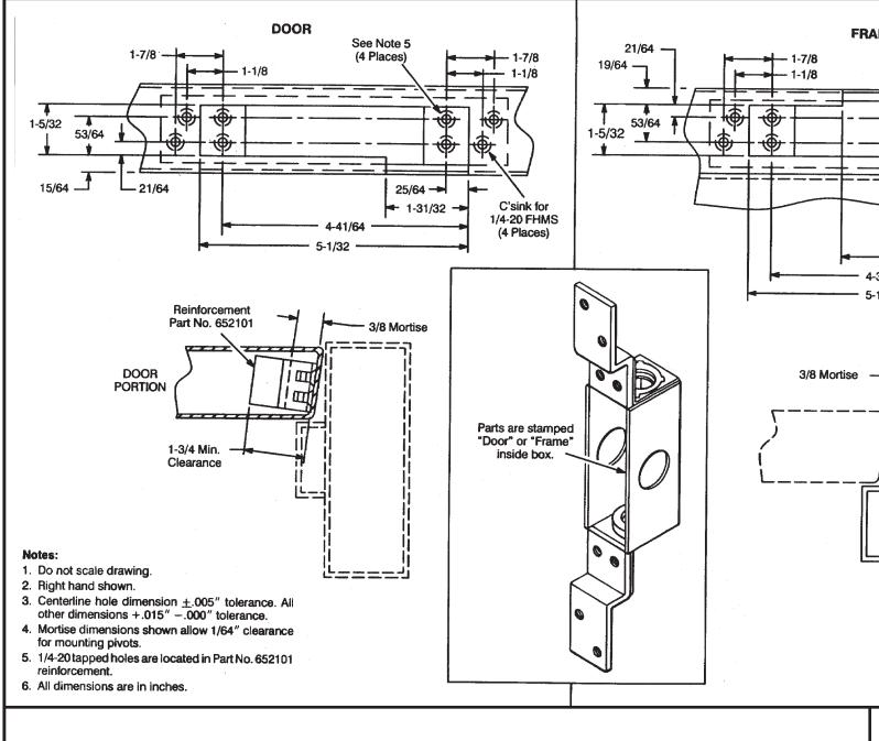
EM19U Intermediate Pivot 3/4" Offset Aluminum Door and Frame Preparation
