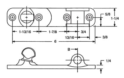
**HAND:** To change the hand of the holder, remove screws at "G" and reverse arms. Be sure screws are tight after reassembling.
