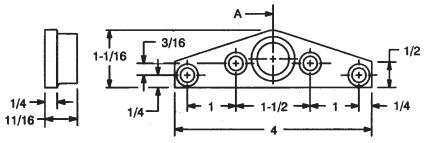
Locate door bracket on door as noted above. Thumb piece must be located towards door pivot. Install door bracket with mounting holes 13/16" down from stop strip as shown on opposite side of page.
