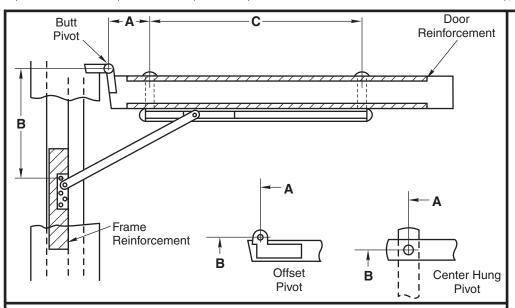
5. Install channel on door with "A" dimension sex bolt. Locate "C" dimension sex bolt hole making sure that channel is horizontal and parallel with stop strip. Drill 1/2 (12.7) dia. sex bolt hole and finish installing holder.
