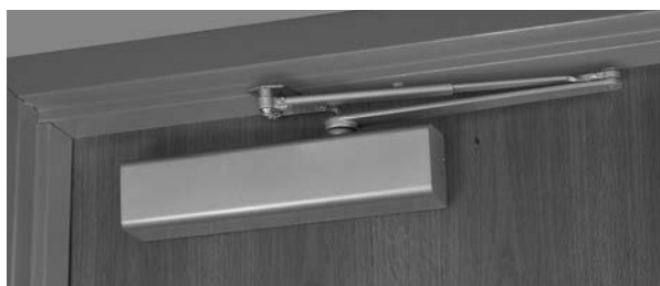
Parallel Arm - allows closer to be installed 1/2" (13mm) higher up on door than standard parallel arm application.
