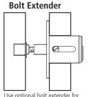
Use optional bolt extender for excessive gaps in bypassing doors.
