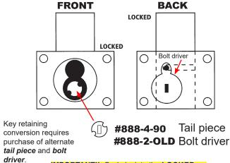
IMPORTANT!! Cycle lock to the LOCKED POSITION before inserting the core.
