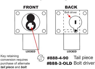
Standard FSIC Cylinder Vertical-Hand (VH) Key Retaining
