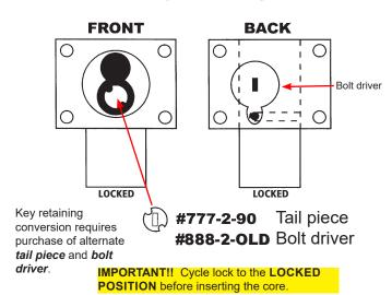
Primus/Everest FSIC Cylinder Vertical-Hand (VH) Key Retaining
