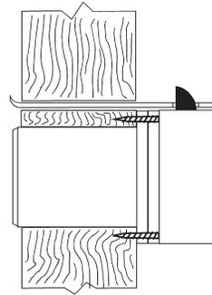
**Note:** Strike must be lined up so that dead lock portion of latch is depressed when drawer is closed.
