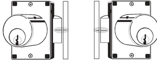
**Strike installation:** Line up center mark on latch with center mark on strike for correct strike placement.
