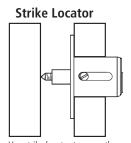
Use strike locator to correctly mark location to install strike.
