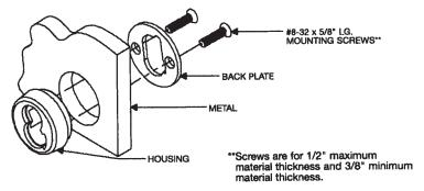
**Note:** Material thickness can be changed by using an "O" ring or changing the screw length.
