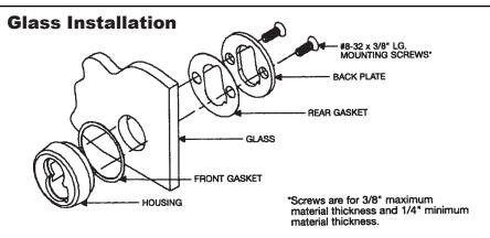
**Note:** Material thickness can be changed by using an "O" ring or changing the screw length.
