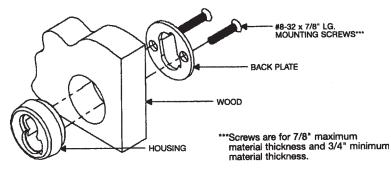
**Note:** Material thickness can be changed by using an "0" ring or changing the screw length.
