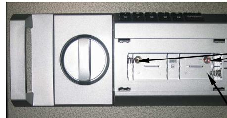
Battery cover and batteries removed. Remove the two housing screws. Carefully allow the housing to hang down and expose the key cylinder.
