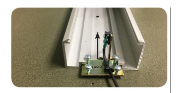
• Depress pushpad and slide until REX triggers on the pushpad, secure REX bracket by tightening all (4) screws.
