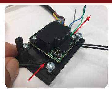
B. Pull wires thru and line up REX switch with REX post with REX arm facing outwards.
