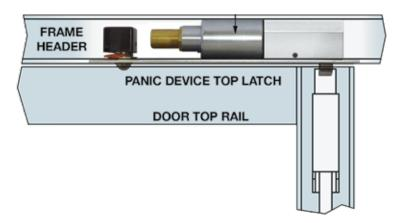
Top Latch Release for Dor-O-Matic and Kawneer Vertical Rod Exit Devices. The PD2090A PanicLok permits access control and remote timer control of narrow stile glass doors equipped with Dor-O-Matic or Kawneer concealed vertical rod exit devices.
