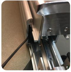
2. Once the pad had been re-installed there should be no gap between the screw holes for the head assembly and the REX.
