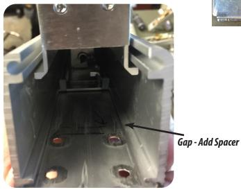
3. With switch installed, flip device over & reinstall (4) screw attaching head assembly to rail housing.
