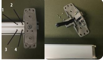
**3.** Remove (1) screw from back of baserail then slide push pad off rail housing.
