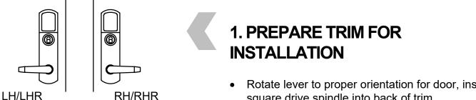
Rotate lever to proper orientation for door, install square drive spindle into back of trim.
