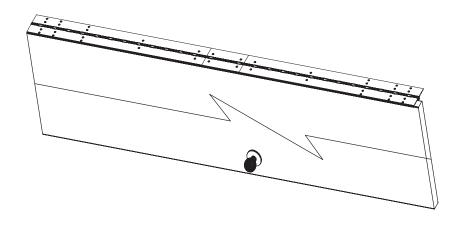
E. Install the lower section of the serviceable / removable hinge per general installation instruction steps No. 2 and 3.
