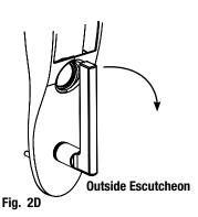
IMPORTANT: Use caution when threading outside lever to bushing. Lever should not come in contact with the surface of the escutcheon.
