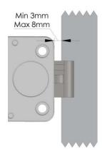
The distance between the SpringBolt lock and the locking edge must be between a minimum of 3 mm and a maximum of 8 mm.
