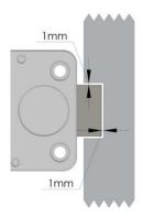
In the locked position, there should be approximately 1 mm clearance between the lock bolt and the cavity in the blocking bar of the boltwork. The bolt must be able to move freely without force being applied to it.
