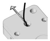
Connect the keypad cable to the lock connector "ENT", making sure it is fully inserted and locked. Any alarm interface or battery holder will be connected to the lock connector "BAT". To remove the cable, bring the connector upwards and carefully pull it out.
