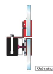
Bracket Kit for Mounting Mini Magnetic Lock on Full Glass Door and Frame.
