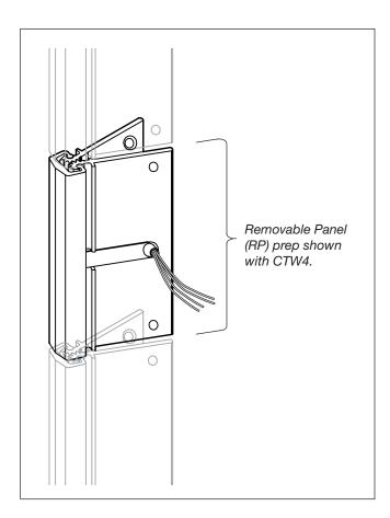
**PREP:** SELECT geared continuous hinges can be prepared with removable hinge leaf panels to allow easy access and service of electrical components without removing the door.
