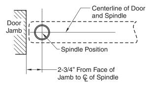
A. Measure 2-3/4" out from door jamb on centerline of door. This is the location of the spindle center.
