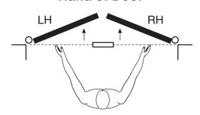
Face a door swinging open away from you. If it opens to the right, it is right hand. If it opens to the left, it is left hand. NOTE: This product allows door to swing in both directions.
