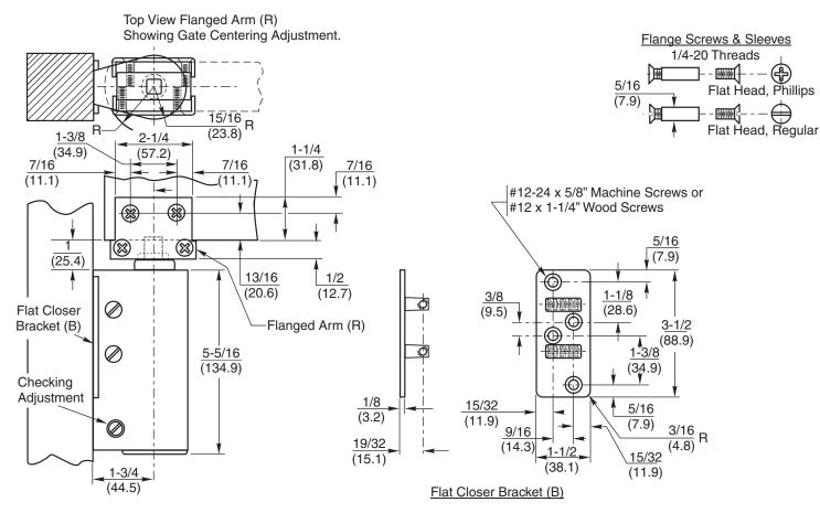
DO NOT SCALE DRAWING Dimensions given in inches (mm).
