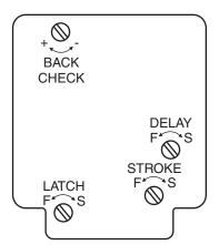
Closing speeds can be adjusted to suit local conditions and requirements. Label on closer face designates the purpose of each adjustment screw. Adjustments are for speed control.
