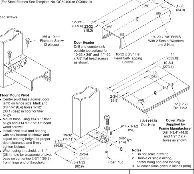
608 Series Concealed Overhead Door Closers **Double or Single Acting for Aluminum Doors & Frames** Center Hung, Side Loading
