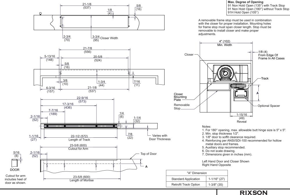
**Model 91 Overhead Concealed Closer Butt Hinge, Metal Frame**
