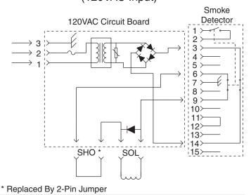
All wiring diagrams are shown with circuits energized in stand by mode.
