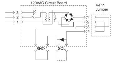
\* Replaced By 2-Pin Jumper
