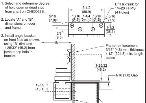
4. Install channel on door with "A" dimension and 19/32 (15.1) from top of door. Locate "C" dimension sex bolt hole making sure that channel is horizontal and parallel with top edge of door. Drill 1/2 (12.7) dia. sex bolt hole and finish installing holder. Install control knob on channel as shown. Install jamb bracket to angle bracket.
