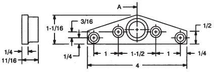
3. Locate door bracket on door as noted above. Thumb piece must be located towards door pivot. Install door bracket with mounting holes 13/16" down from stop strip as shown on opposite side of page.
