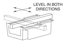
A. For floor plate application: the top of the closer case (or cement case as both are the same level) is set 1/16" below finished floor.
