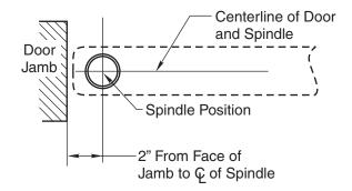
A. Measure 2" out from door jamb on centerline of door. This is the location of the spindle center.
