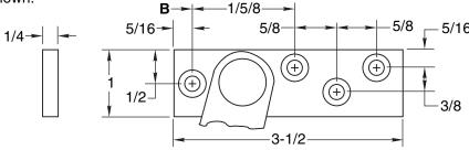
3. Locate "A" and "F dimensions on centerline of door and mortise 3/4" deep for channel. 1/16" head clearance shown. Coordinate the arm and rail cutout dimensions if head clearance varies.
