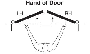
Face a door swinging open away from you. If it opens to the right, it is right hand. If it opens to the left, it is left hand. NOTE: This product allows the door to swing in both directions.
