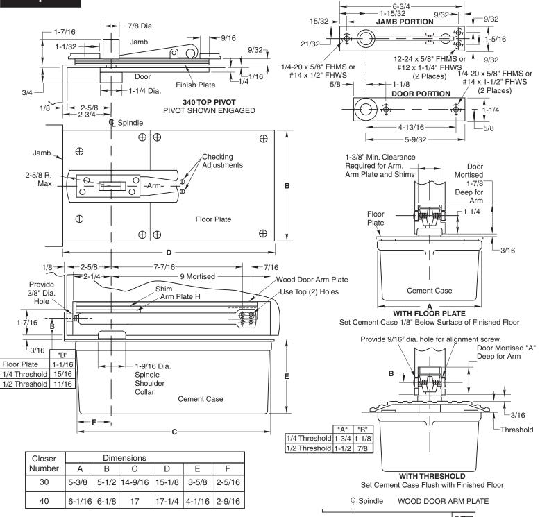
Conversion from inches to metric: inch x 25.4. Suitable reinforcing by others.
