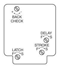
Closing speeds can be adjusted to suit local conditions and requirements. Label on closer face designates the purpose of each adjustment screw. Adjustments are for speed
