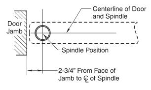
A. Measure 2-3/4" out from door jamb on centerline of door. This is the location of the spindle center.
