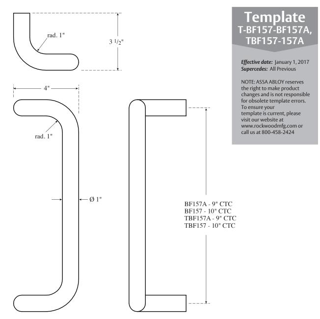
Material Brass, Bronze, Stainless Steel (solid or tube) Alum (solid only) This item can be mounted to glass, metal or wood doors. Back to back is by type 16 or 18. Thrubolt is by type 1, 12, or 15. Concealed is by type 17.
