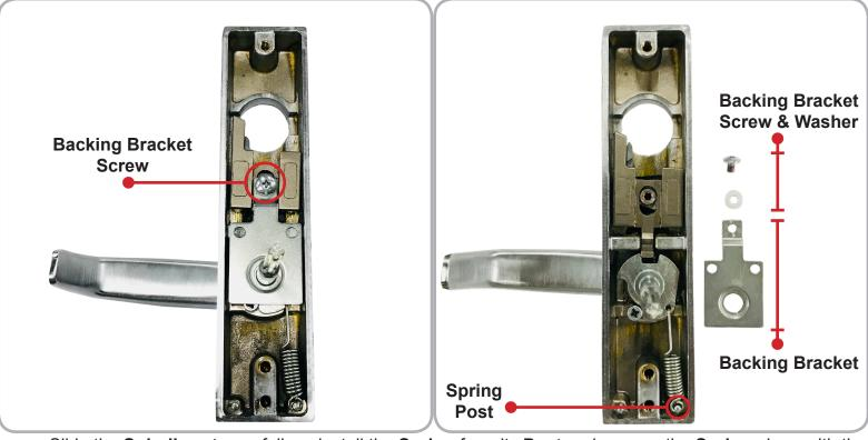
Slide the **Spindle** out, carefully uninstall the **Spring** from its **Post** and remove the **Spring** along with the **Spindle Plate**. Remove the **Retaining Screw** and place the **REE Switch Mounting Bracket** over the Retaining Screw hole, then reinstall the screw.
