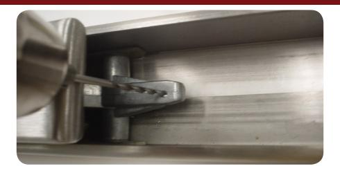
E. Test Rex switch for proper operation and adjust if neccessary
