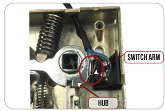
**5.** Line up REX Bracket with existing hole underneath locking hub & secure REX switch.
