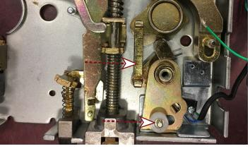
REPLACE COVER. IF NEEDED PULL ON ANTI-PIC & PUSH LATCHBOLT TO HELP CASE SLIP TOGETHER. TEST THAT LATCHBOLT & ANTI-PICK
