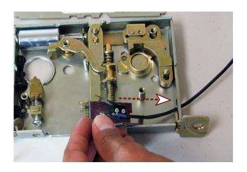
F. REPLACE HUB CENTER SPRING ASSEMBLY (5). LINE UP & PLACE OVER POSTS SO (5) LIGHTLY RESTS ON SWITCH.
