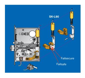
Convert Mechanical Lock into Electric Access Controlled Lock. **SDC SK Field Electrification Kit** for Schlage L9000, mortise locks allows for fast electrification of existing locks in the field. Failsafe and Failsecure options are easily selected and can be changed in the field to suit any need. Optional Request-To-Exit kit provides indication of inside lever operation for alarm shunt, remote annunciation or CCTV activation.
