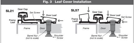
**NOTE:** For inswing applications, reverse position of barrel nut and shoulder screw so that the shoulder screw is on the secured side of the door.
