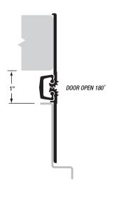
**MATERIAL:** Extruded 6063 T6 aluminum alloy with self-lubricating polyester thrust bearings.
