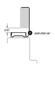
**MATERIAL:** 14 gauge 304 stainless steel barrel with 3/16" diameter 304 stainless pin. Long-life nylon medical bearings.
